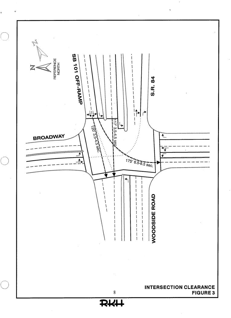
ramp. The clearance times were measured using a stop watch and the range of observed times are shown on Figure 3.
