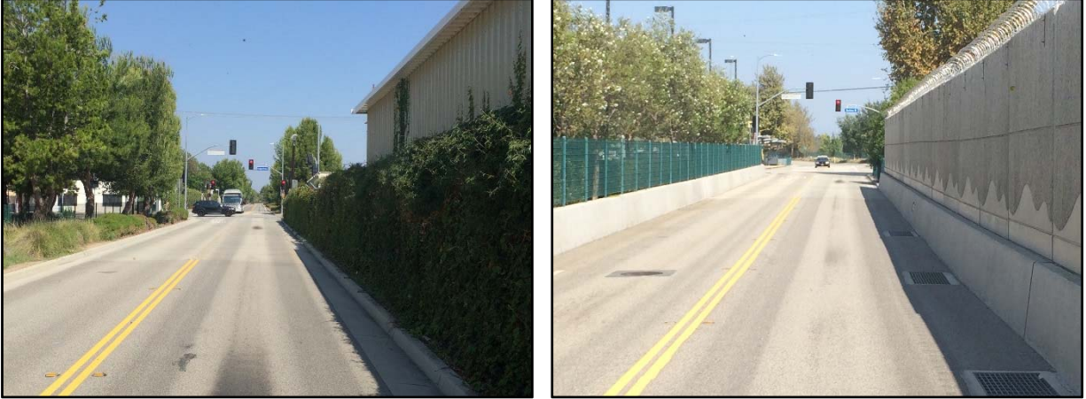
Exhibit 2: Sight distance constraints due to landscaping, buildings, and walls
