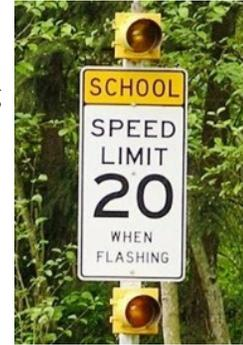
This sign provides a specific indication to motorists as to when the lower speed limit is in effect. Research has shown that the flashing beacon is highly effective in reducing speeds in school zones and increasing compliance. However, this sign is currently not permitted for use in California.
